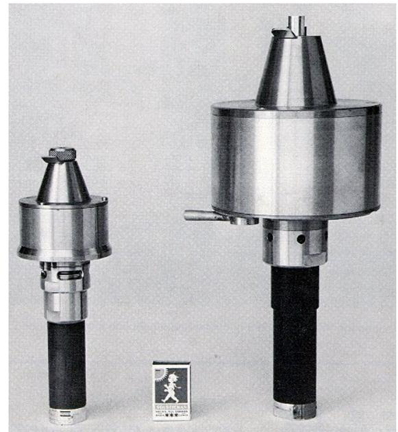
The centrifuge is at present manufactured in a small (H-10, total flow capacity 100 l/h) and a medium (H-33, total flow capacity 300 l/h) sized version. The smaller version (H-10) can be fitted with different heads, consisting of a mixer unit, flow meters and necessary valves to make a mixer-(centrifugal)settler unit. The larger (H-33) centrifuge is used in the AKUFVE-110 instrument.
