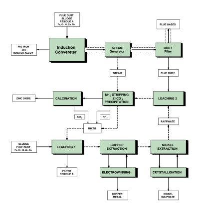
feasibility of The а pyro/hydro-metallurgical **UDDAMAR** process as a centrally located recovery plant for the treatment of oxidic and hydroxidic metal containing waste from steel and metal works, including the plating industry, has been investigated some vears ago in Sweden. The process, shown in the figure, is based on the use of the **UDDACON** induction converter and the AmMAR wet process technology
